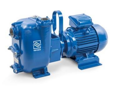
**Product Data** Suction port Threaded - 1 1/2" ISO 228 (BSP) Delivery port Threaded - 1 1/2" ISO 228 (BSP) Qmax 25 m<sup>3</sup>/h - 416 l/min (110 USgpm) Hmax 37 m (121 ft) Solids handling 11 mm (0.4 ") Motor power 4 kW - 5,5 HP Motor type **IEC** standard Winding for inverters **Cast iron frame** Motor brand WEG W22 Premium Weight 90 kg
